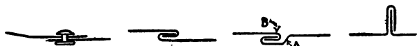
FIG. 175. Riveted Lap Seams for Sheet Metal. FIG. 176. Common Lock Seam for Sheet Metal. FIG. 177. Groove Seam for Sheet Metal. FIG. 178. Common Standing Seam for Sheet Metal.
